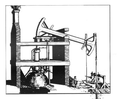
piston inside a cylinder. Water sprayed into the bottom of the cylinder was heated from below, creating steam. The steam created a vacuum, which forced the piston to rise. The piston was attached to one end of a great wooden beam that resembled a giant seesaw. As the piston rose, it forced the beam up on one end and down on the other.
