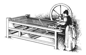
to spin eight threads simultaneously. Later models increased the number of simultaneously produced threads to 100! Acceptance of such a device by cloth workers was slow. (In fact, Hargreaves, too, had his house sacked and his first spinning jenny burned by angry spinners fearing for their jobs.)
